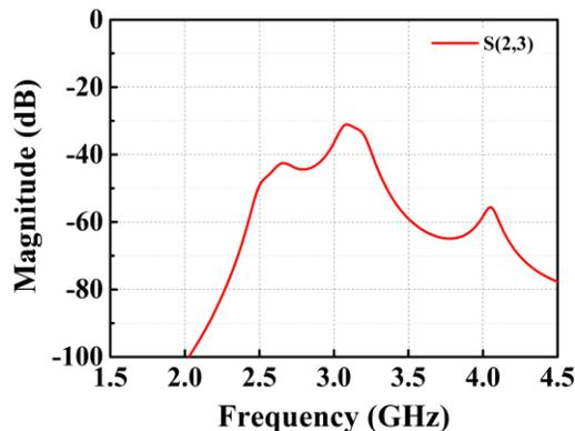
**Figure 7. Simulated result isolation of the proposed diplexer**
