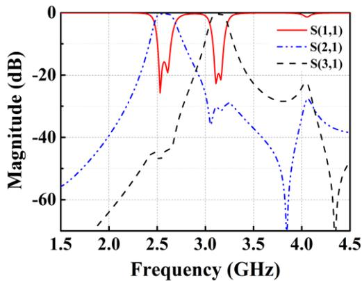
**Figure 6. Simulated result insertion losses and return loss of the proposed diplexer**
