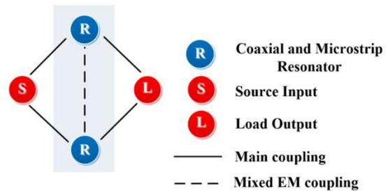
**Figure 2. Coupling structure for the proposed hybrid coaxial and microstrip resonator**
